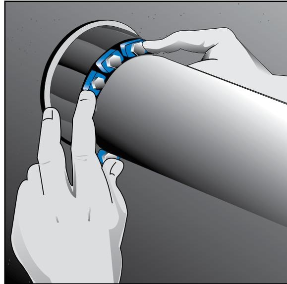
2. Slide the assembly into the space between the pipe and wall.
