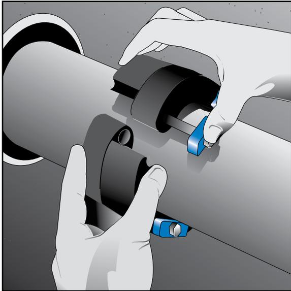
1. Wrap the belt around the pipe. Then connect the first and last links. The proper size and number of links can be found in the catalog.
