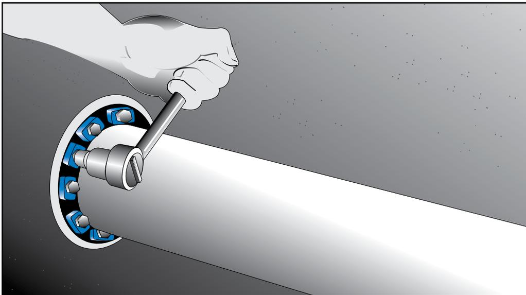
3. Gradually and sequentially tighten the bolts. Tighten each bolt 2-3 turns making 5 to 9 passes completely around the pipe. Do not cross tighten. The PipeSeal links expand to create a gas and water tight seal.
