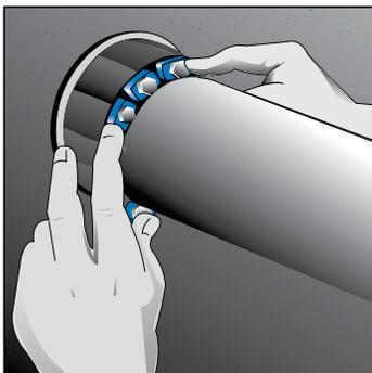
Use a light solution of soapy water as lubricant if needed.
