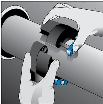
4. For larger sizes, begin inserting the assembly at the 6 O'clock position and push the remaining seal in on both sides as you move up towards the 12 O'clock position.
