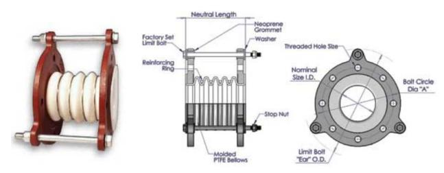
The Teflex expansion joints are composed of unreinforced PTFE and come standard with iron 150# drill flanges. Stainless flanges are available as an option. They are available in 2, 3, or 5 convolutions of varying movements. The 5-convolution joint shown here is sometimes referred to as a "bellows". The 5 – convolute Teflex is not rated for vacuum service.
